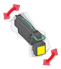
**6** Remove the red packing strip from the new cartridge.
